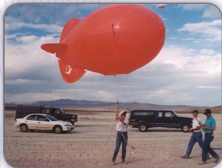
Blimps were used to loft sampling equipment into the cloud of combustion gases immediately after detonation of the missiles.
